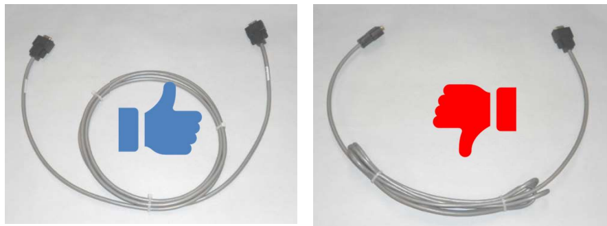
Figure 6. Proper cable slack take-up.
